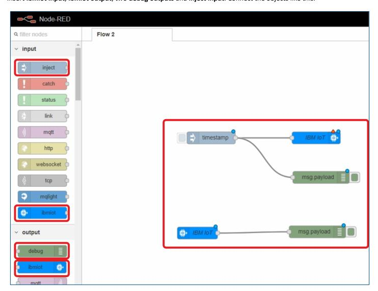
With the inject input we will send **DPA commands** to the MQTT broker on the IBM Cloud and our UP board will collect them from there. We will send the commands to the debug window as an output, as well. We will receive all messages from the MQTT broker and they will be displayed in the debug window.
