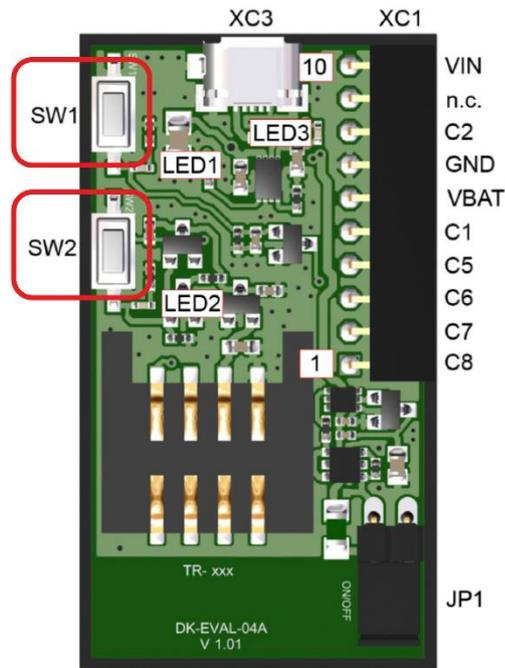
**Caution:** SW2 must be pressed always when you are plugging or unplugging the transceiver to/from the SIM connector.
