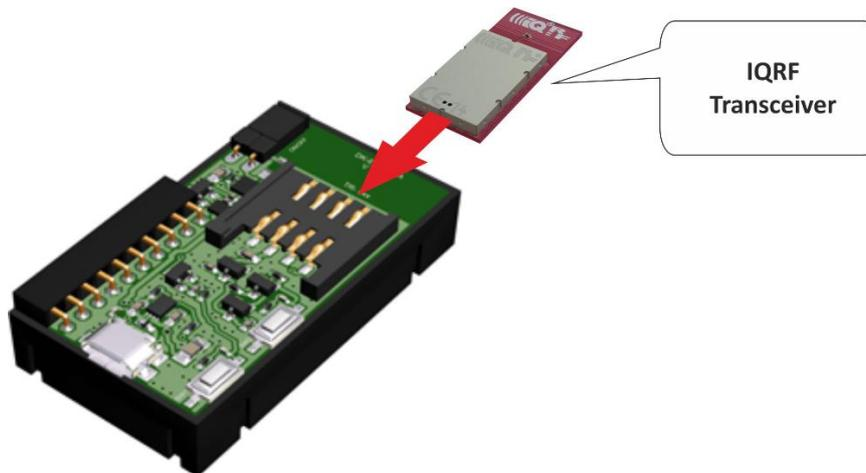
Press and hold the SW2 button (Reset button) on a CK-USB or DK-EVAL always when you are plugging an IQRF transceiver to or you are unplugging it from the SIM connector. Be sure you connect an IQRF transceiver into a CK-USB or DK-EVAL in the right direction (the antenna is outside the SIM connector).
