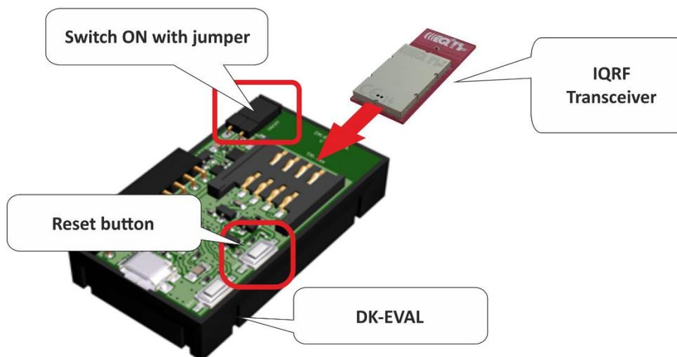
If the red LED on the IQRF transceiver is flashing, it means it has no previous bonding information stored. If this is not the case, you must unbond the node. We will do it here manually.
