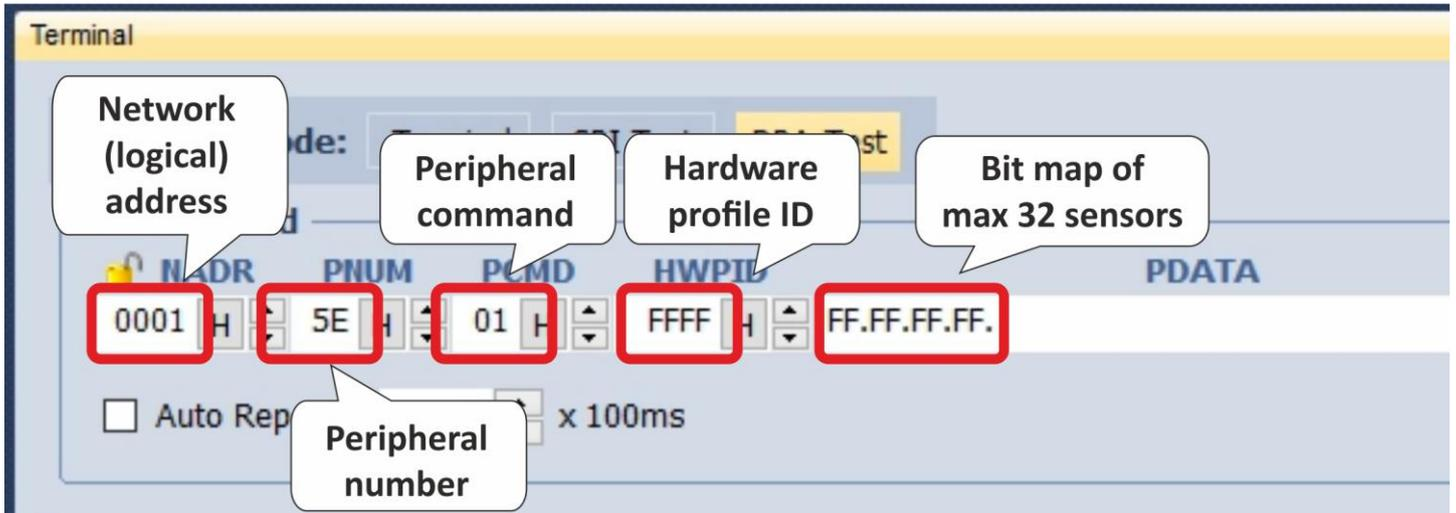
Send the command and see the ongoing communication in **Terminal Log**.
