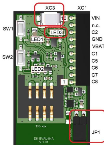
**SW1** is a **User** pushbutton which is connected to pin C5 of the transceiver. It will be used here for bonding (adding to a network) in next steps.
