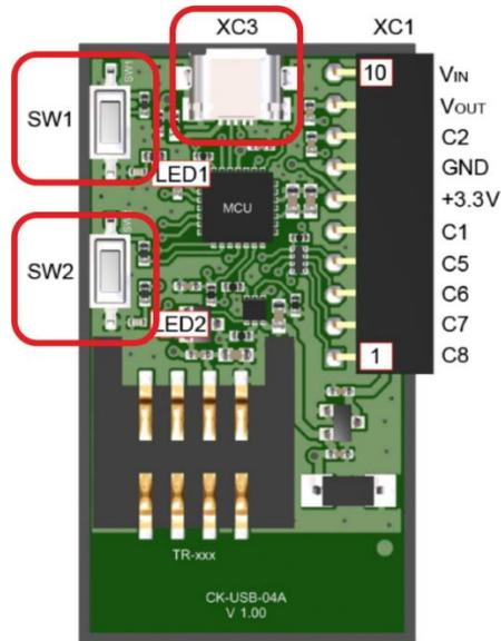
**Caution:** The IQRF transceiver can be plugged into / unplugged from the SIM connector while powered off only. The SIM connector is not powered while the SW2 pushbutton is held. Press and hold it always when you are plugging an IQRF transceiver to or you are unplugging it from the SIM connector of CK-USB.
