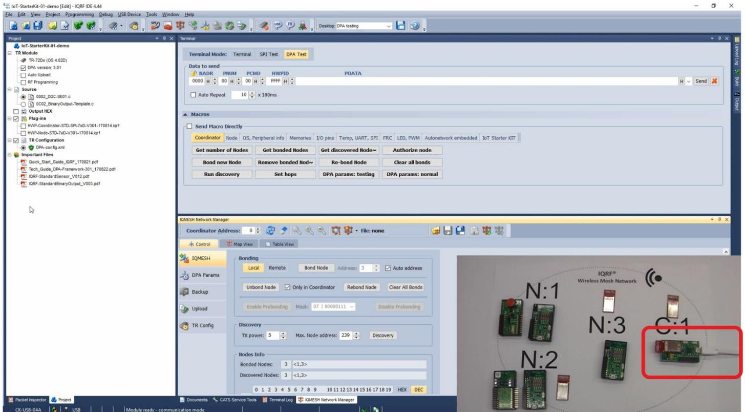
On the left-hand side, you double-click on the configuration. Don't change the selected channel 52, because all devices you will connect to the network later will have the default channel 52 as well.
