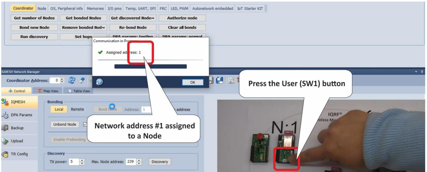
Bond the transceiver with the Custom DPA Handler for communication with relays as a node number 2 following the same procedure. The last transceiver will be bonded as number 3. You can see the current network in the **Map View**.
