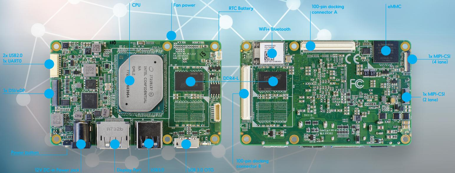
UP Core Plus is a credit card-sized board with high performance and low power consumption which features of the latest the Intel® Atom™ x5 / x7 / Celeron / Pentium processor 64 bits up to 2.5 GHz.
