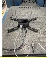
4. Sinusoidal Vibration Test/ Random Vibration Test: Y axis
