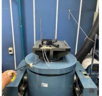
Sinusoidal Vibration Test/ Random Vibration Test: Z axis
